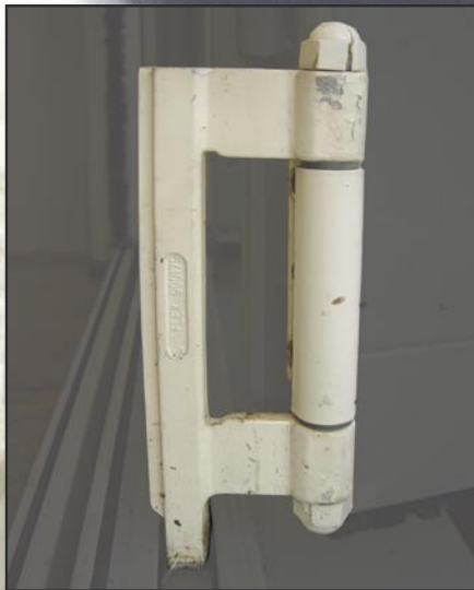
competitors powder coated alloy hinge, weathered in a non marine environment
